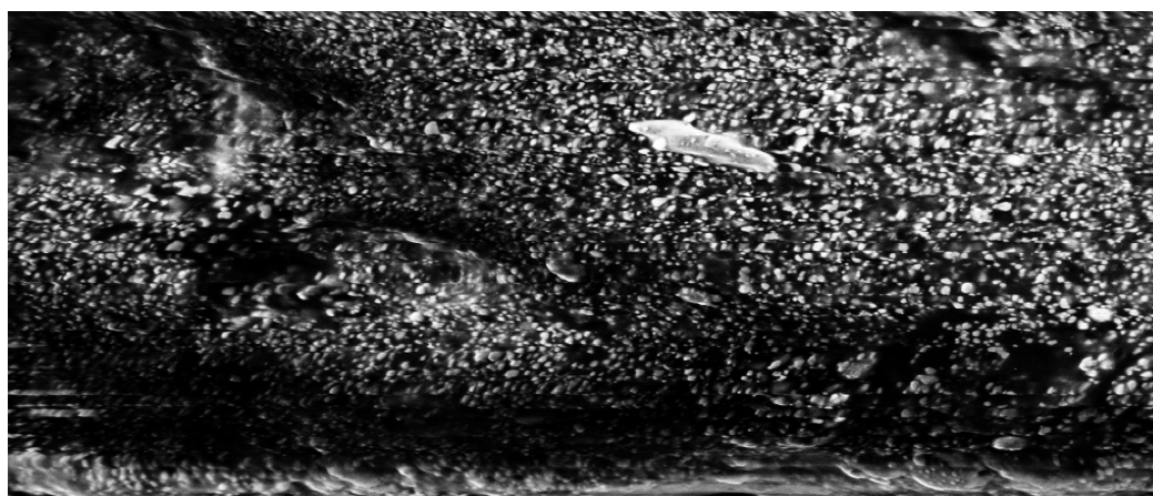
Figure 4 SEM image of synthesized silver nanoparticles of Ficus auriculata
