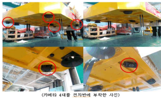
Photo 1: Prototype of EMS 3point Trolley with having Installed 4 Monitoring Cameras
