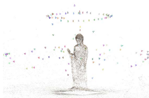
Figure 3: Structure-from-motion Reconstruction Showing the 3D Point Cloud and All of the 121 Camera Poses
