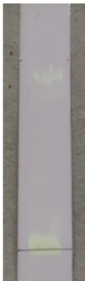
Figure 5 DPPH Bio-Autography by TLC
