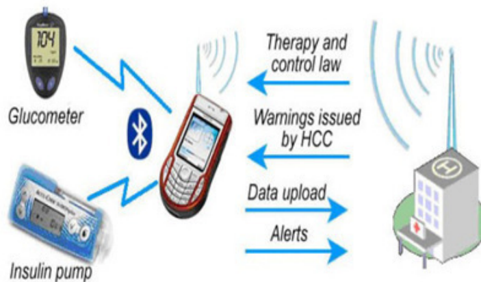
Figure 4.1 Mobile Architecture for Glucose Monitoring
