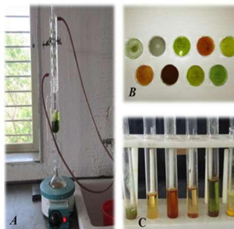
Figure 2 A =Extraction by Soxhlet B = Extraction in different Solvent C = Phytochemical Test
