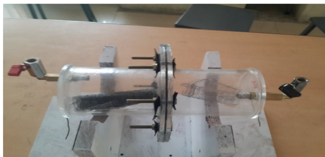
Figure 6 Microbial Fuel Cell (MFC) Setup
