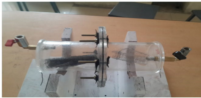
Figure 6 Microbial Fuel Cell (MFC) Setup
